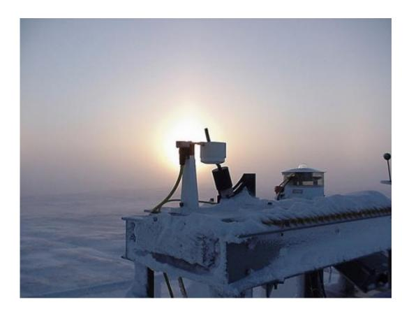
Caught in the early morning light, the multifilter rotating shawdowband radiometer instrument takes measurements of direct and diffuse sunlight in Barrow, Alaska. Now that PNNL scientists have devised a new method for screening out the thin clouds prevalent at this Alaska site, those measurements will be much more effective. Credit: ARM Climate Research Facility.
