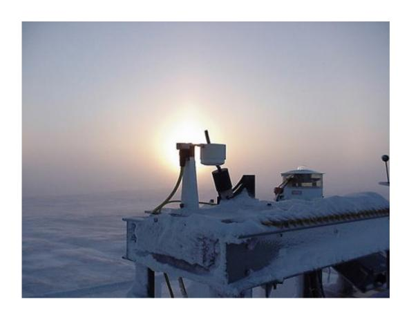
Caught in the early morning light, the multifilter rotating shawdowband radiometer instrument takes measurements of direct and diffuse sunlight in Barrow, Alaska. Now that PNNL scientists have devised a new method for screening out the thin clouds prevalent at this Alaska site, those measurements will be much more effective. Credit: ARM Climate Research Facility.
