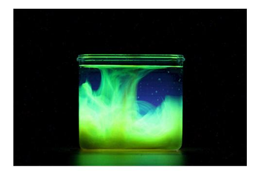
Long exposure image of Cherenkov emission and induced fluorescence from Fluorescein dissolving in water during irradiation from a therapeutic LINAC beam. Credit: Adam Glaser.
