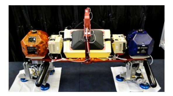
The SPHERES-Slosh hardware used aboard the space station will help researchers study the movement of fluids in microgravity. This may assist with designing new, more efficient fuel tanks. Credit: Florida Institute of Technology/Dr. Daniel Kirk
