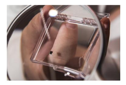
The small device seen under a magnifying glass is an array of microcantilevers. Rice University scientists are decorating the array with peptides that capture strains of salmonella. The technique could make the detection of pathogens
