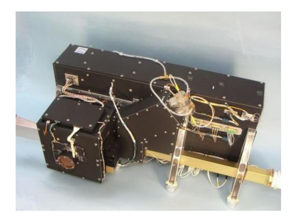
The COSIMA dust analyzer will investigate cometary material from the atmosphere of 67P/Churyumov/Gerasimenko. The instrument's main task here is to identify organic molecules. Credit: MPE/MPS
