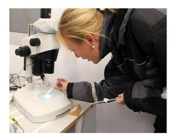
Ph.D student Kine Nilssen conducting an experiment on ice adhesion. Provisional data indicate that ice binding is significantly weakened when salt is present, although so far, no-one knows why. Credit: SINTEF
