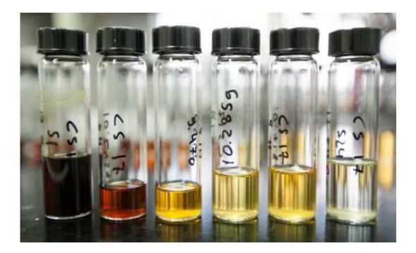
The flow-through reaction setup progressively dissolves biomass producing fractions that are rich in (from left to right) lignin monomers, hemicellulose and cellulose-derived sugars. Credit: Matthew Wisniewski/Wisconsin Energy Institute
