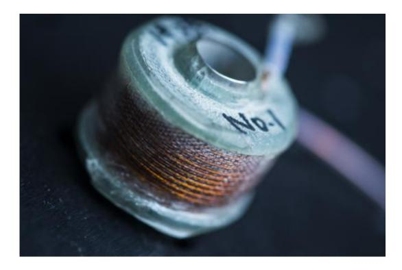
A palm-sized coil is the heart of RAMBO, a Rice-built tabletop system to expose experiments to high magnetic fields. The coil developed by Hiroyuki Nojiri at Tohoku University in Japan provides a pulsed field of up to 30 tesla and allows for the collection of data at close range. Credit: Jeff Fitlow/Rice University
