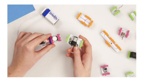
An example of the Bits modules. Here, a power source (blue) connects to a button (pink) that will trigger a motor (green). The orange modules to the side are extending wires. Credit: : LITTLEBITS
