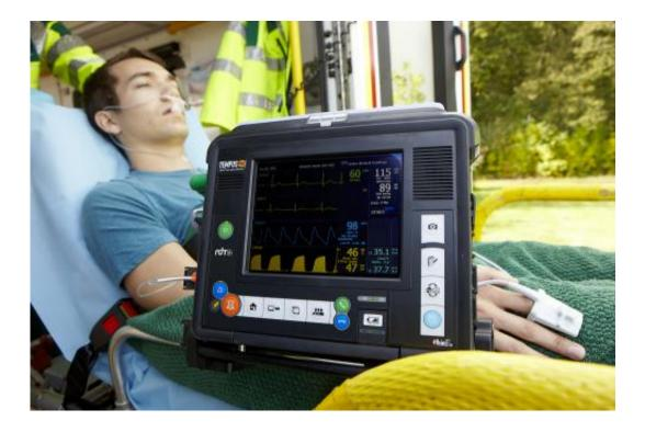
The Tempus Pro has been developed by Remote Diagnostic Technology (RDT) in the UK, with funding from ESA's Advanced Research in Telecommunications Systems programme. The unit combines the diagnostic facilities found in standard hospital vital signs monitors with extensive two-way communications, packaged in a compact, robust, highly portable unit that can be tailored to user needs with the use of external devices. It has GSM (3G), GPS, wi-fi, bluetooth
