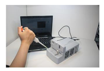
Analyses of liquid samples that once required a full-sized laboratory can now be completed on a disposable plastic chip equipped with narrow fluidic channels and tiny sensors. Credit: A\*STAR Institute of Materials Research and Engineering
