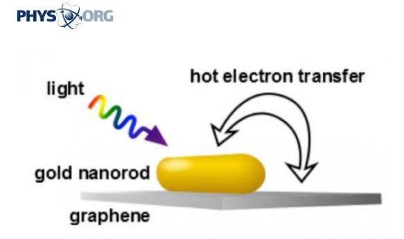
Rice University researchers determined the amount of time it takes electrons generated by plasmons in a gold nanorod to transfer to a sheet of graphene through spectroscopic analysis of hundreds of particles. The research will help scientists strategize on ways to gather and store electrons from plasmonic particles. Credit: Anneli Hoggard/Rice University
