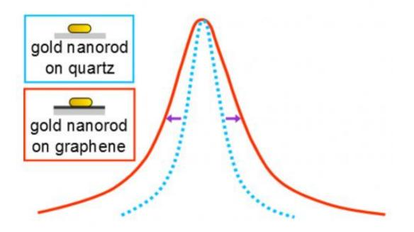
The plasmon resonance of gold nanorods on graphene is broadened compared with gold nanorods on quartz, according to a new study by Rice University scientists. The additional peak width was attributed to excited electron transfer between gold nanorods and graphene. Credit: Anneli Hoggard/Rice University
