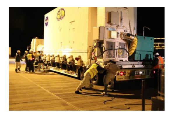
GPM on its last truck. On the back of the shipping container sits the Environmental Control Unit (left), as well as its generator (green on the right). The ECU has heaters and air conditioners to regulate temperature and humidity as well as filters on the air vents to keep out any contaminants. Credit: NASA Goddard/Michael Starobin
