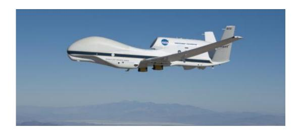
NASA Global Hawk 872 carries the Hawkeye sensors on wing-mounted pylons during a checkout flight of ATTREX instruments. Credit: NASA / Tom Miller
