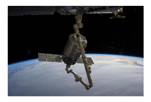
The Orbital Sciences Corp. Cygnus commercial cargo craft attached to the end of the Canadarm2 robotic arm of the International Space Station is photographed by an Expedition 38 crew member during rendezvous and berthing operations on Jan. 12, 2014. Credit: NASA
