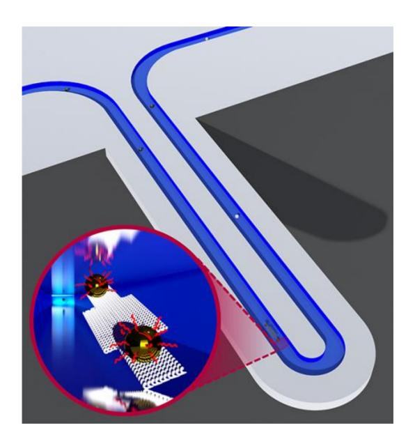
The illustration shows a suspended nanochannel resonator (SNR), which can directly measure the mass of individual nanoparticles with single-attogram precision. The inset shows a depiction from inside the embedded fluidic channel, while a DNA-origami gold nanoparticle assembly is passing through the
