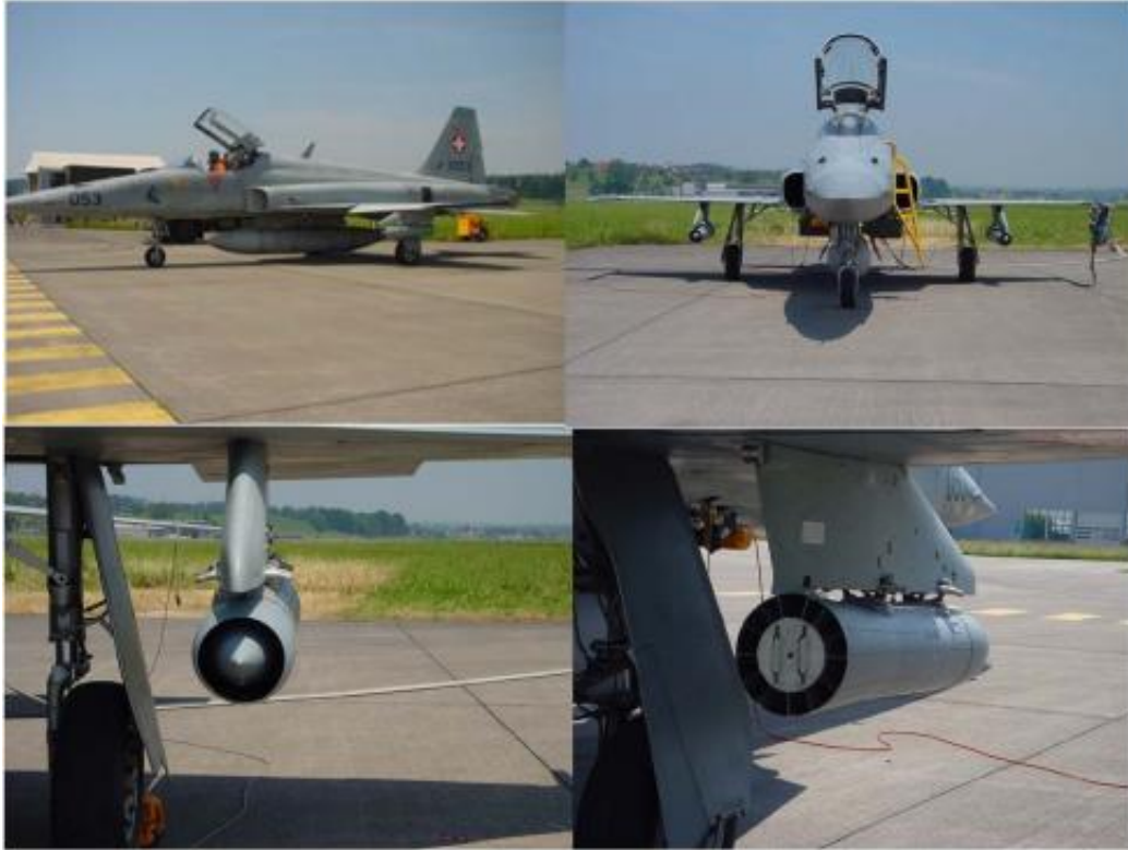
The aerosol collection devices mounted on the wings of a Tiger (F5E/F), aircraft of the Swiss Air Force. Credit: Swiss Federal Office of Public Health
