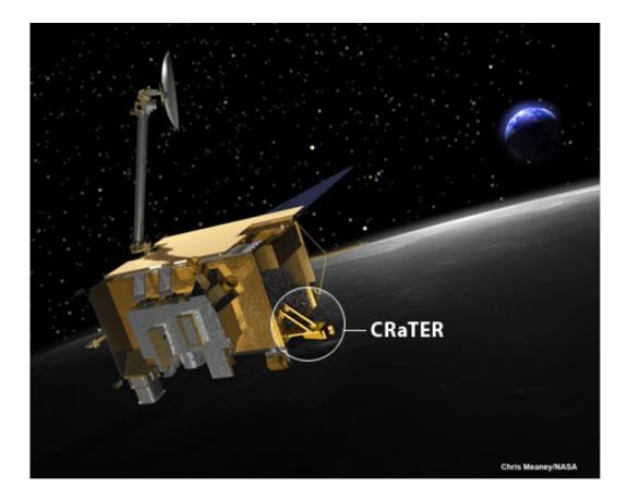
The Cosmic Ray Telescope for the Effects of Radiation, or CRaTER, on NASA's Lunar Reconnaissance Orbiter has six detectors to monitor the energetic charged particles from galactic cosmic rays and solar events. Credit: NASA/GSFC
