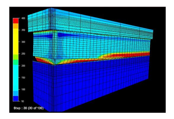
New, user-friendly modelling tools put the aluminium industry in a position to simulate the outcomes of choosing certain alloys and casting parameters, thereby increasing processability. Credit: SINTEF
