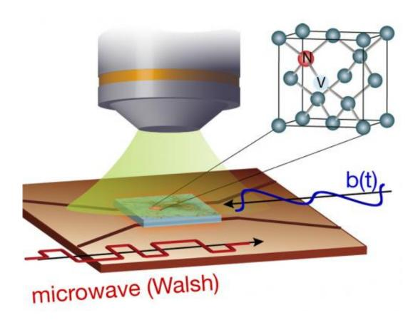
A single nitrogen-vacancy (N-V) center in diamond (right, inset), optically initialized and readout by confocal microscopy, is manipulated with coherent control sequences (red line) of microwave pulses. This measures the arbitrary profile of time-varying magnetic fields radiated by biological sources (or by artificial sources in the researchers' proof-of-principle experiment). Credit: Paola Cappellaro
