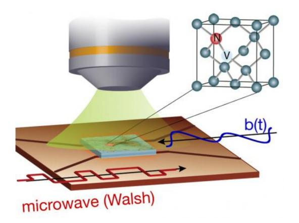
A single nitrogen-vacancy (N-V) center in diamond (right, inset), optically initialized and readout by confocal microscopy, is manipulated with coherent control sequences (red line) of microwave pulses. This measures the arbitrary profile of time-varying magnetic fields radiated by biological sources (or by artificial sources in the researchers' proof-of-principle experiment). Credit: Paola Cappellaro
