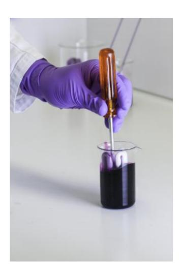
A new method developed at Empa allows scientists to determine not just the quantity of bound mercury in an energy-saving lamp, but also the amount of mercury vapour. To do this the lamp is immersed in a solution of potassium permanganate and its glass envelope broken open. The chemical solution is sucked into the broken lamp where it immediately reacts with the vaporized mercury, preventing it from escaping.
