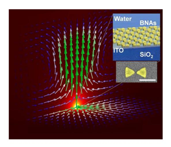
This is a depiction of the fluid convection (arrows) overlaid on the background temperature distribution produced by the BNAs and ITO. The inset shows the BNA geometry with a (false color) scanning electron microscope image of a single bowtie; scale bar is 200 nm. Credit: University of Illinois
