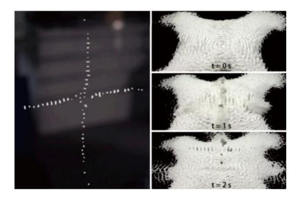
(left) Levitation and manipulation of particles. (right) Scooping up and holding particles. Credit: arXiv:1312.4006 [physics.class-ph]
