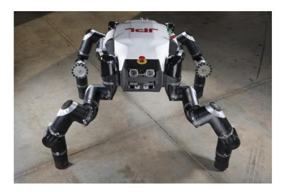
The Jet Propulsion Laboratory's official entry, RoboSimian, awaits the first event at the DARPA Robotics Challenge in December 2013. Also known as "Clyde," the robot is four-footed but can also stand on two feet. It has four general-purpose limbs and hands capable of mobility and manipulation. Credit: JPL-Caltech
