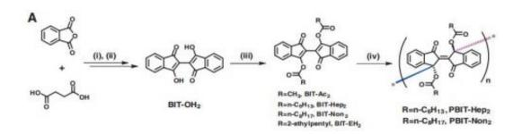
Synthetic route to monomers and polymers. Reaction conditions: (i) melting reaction, potassium acetate, 220°C, 2 hours; (ii) methanol, sodium, 60°C, 30 min; (iii) acyl chloride, triethyl amine, dichloromethane, 0°C to room temperature, 3 hours; and (iv) where  $\hbar$  is Planck's constant, n is the frequency, and l is the wavelength of the photon's radiation,  $\hbar$ n, 1 ~ 500 nm. Credit: *Science* 17 January 2014: Vol. 343 no. 6168 pp. 272-277 DOI: 10.1126/science.1245875
