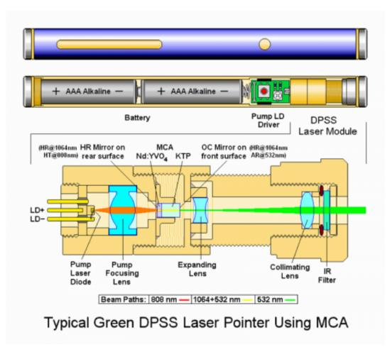
Components of a typical green laser pointer. There are three different wavelengths involved in creating the laser beam. One, at 808 nm, pumps a crystal which lases at 1064 nm, in the infrared. That beam then travels through another crystal which doubles the frequency, cutting the wavelength to 532 nm green. All three wavelengths are emitted, and the pointer's total power output is the sum of these. Credit: Chris Chen, Wikimedia Commons
