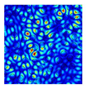
Computed optical light fields in a random laser overlaid on black circles, which represent the nanoholes drilled into a semiconductor quantum cascade laser, to produce a laser pattern with low spatial coherence. Credit: 2013 WILEY-VCH Verlag GmbH & Co. KGaA, Weinheim
