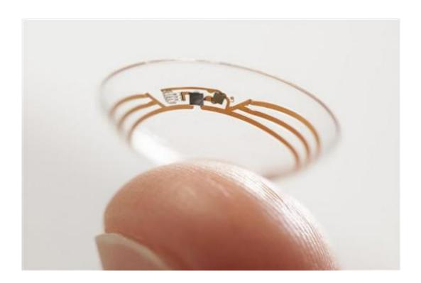
This undated photo released by Google shows a contact lens Google is testing to explore tear glucose. After years of scalding soldering hair-thin wires to miniaturize electronics, Brian Otis, Google X project lead, has burned his fingertips so often that he can no longer feel the tiny chips he made from scratch in Google's Silicon Valley headquarters, a small price to pay for what he says is the smallest wireless glucose sensor that has ever been made. (AP Photo/Google)
