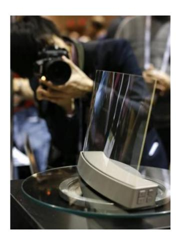
Members of the media photograph a glass speaker called Clio during the International Consumer Electronics Show, Sunday, Jan. 5, 2014, in Las Vegas. The speaker, produced by ClearView Audio uses a single piece of curved millimeter-thick acrylic glass that sits on a dock which vibrates it in a finely tuned way so that it can play music. It works with Bluetooth streaming and with a 3.5 millimeter jack. (AP Photo/Julie Jacobson)
