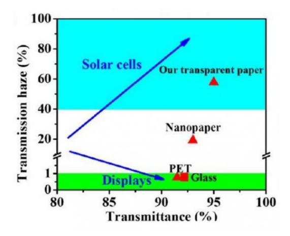
Optical transmission haze versus transmittance for different substrates at 550 nm. Glass and PET are in the green area, which are suitable for displays due to their low haze and high transparency; the transparent paper developed in this work is located in the cyan area, which is the most suitable for solar cells. Credit: Fang, et al. ©2014 American Chemical Society
