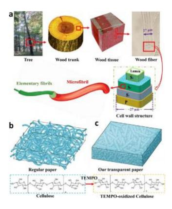
(a) A schematic of the hierarchical structure of a tree in which each structure is broken down to the level of the elementary fibrils. (b) Regular paper with microfibers has a microporous structure that causes light scattering. (c) The new paper is made of TEMPO-oxidized wood fibers to eliminate the micropores and improve optical transparency. Credit: Fang, et al. ©2014 American Chemical Society
