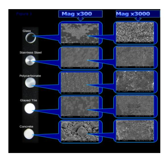
This image shows photos of biofilms on surfaces at low magnification (300) and high magnification (3000) using electron microscope. Credit: Photo courtesy of National University of Ireland, Galway
