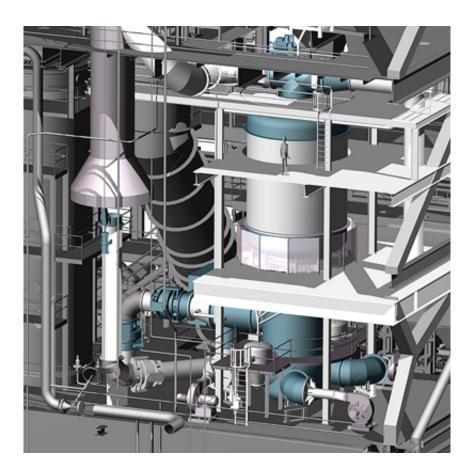
The Siemens Jet Process increases the flexibility of raw material selection on the converter. Oxygen, lime and coal are blown in through bottom tuyeres and a top lance blows hot jet onto the bath. This results in excellent mixing and optimal use of the blown-in coal.
