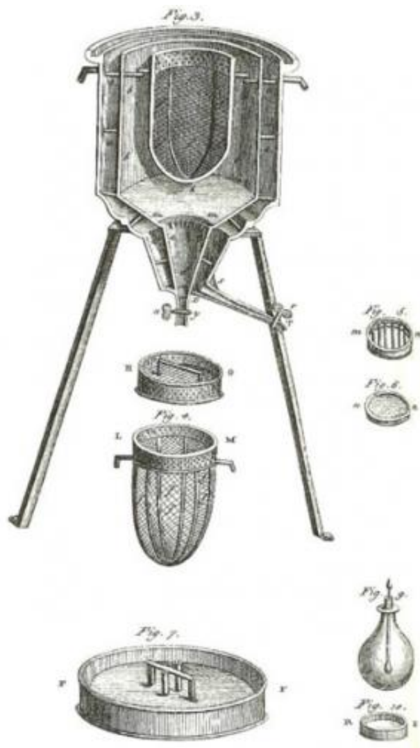
Ice-calorimeter from Antoine Lavoisier's 1789 Elements of Chemistry.
