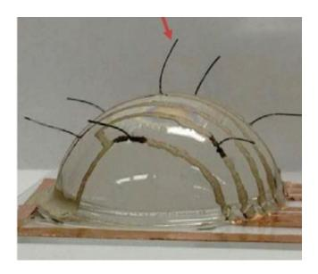
An array of seven vertically placed e-whiskers was used for 3D mapping of the wind by Ali Javey and his group.
