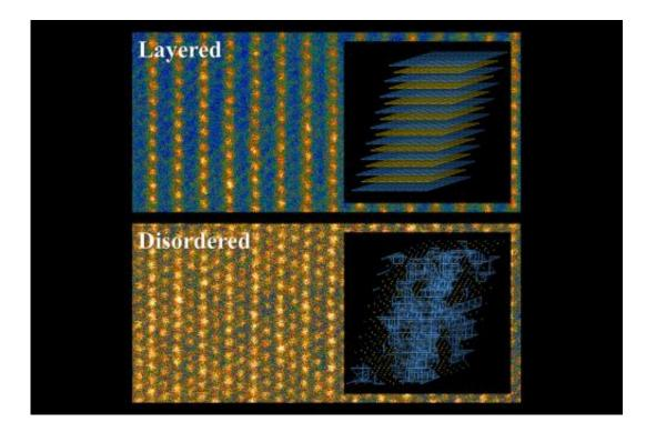
Conventional layered lithium and transition metal cathode material (top) and the new disordered material studied by researchers at MIT (bottom) as seen through a scanning tunneling electron microscope. Inset images show diagrams of the different structures in these materials. (In the disordered material, the blue lines show the pathways that allow lithium ions to traverse the material.) Credit: MIT
