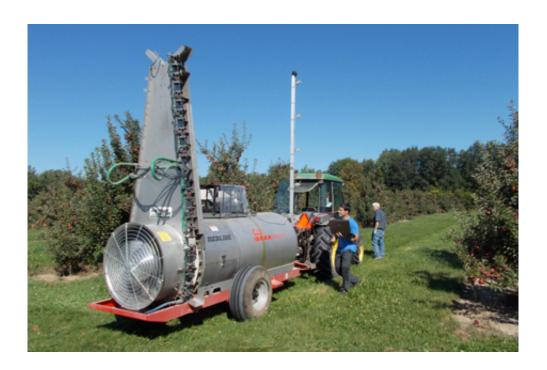
Postdoctoral researcher Jordi Llorens collects data from the prototype precision sprayer, which has ultrasound sensors mounted on the white mast behind the tractor cab and a variable array of spray nozzles mounted at the back of the sprayer.
