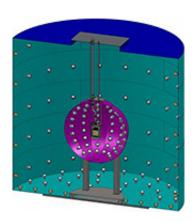
The Darkside-50 experiment consists of three chambers. An argon-filled tank is suspended inside a liquid-filled, room-sized steel sphere, which is suspended in a three-story tank filled with ultrapure water. Researchers are looking for collisions of dark matter and visible matter in the inner chamber, and the outer chambers help distinguish dark matter particles from other particles. Credit: DarkSide-50, Gran Sasso National Laboratory
