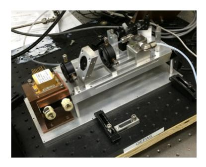
The QEPAS sensor, seen in a Rice University lab, is capable of detecting trace amounts of methane and nitrous oxide. The portable unit was tested during NASA's recent DISCOVER-AQ survey of Houston air quality and proved itself the equal of far larger instruments. Credit: University Laser Science Group
