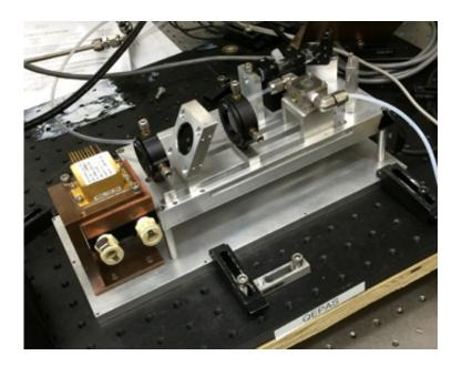
The QEPAS sensor, seen in a Rice University lab, is capable of detecting trace amounts of methane and nitrous oxide. The portable unit was tested during NASA's recent DISCOVER-AQ survey of Houston air quality and proved itself the equal of far larger instruments. Credit: University Laser Science Group
