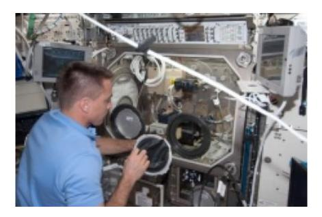
Astronaut Chris Cassidy installs the right glove on the Microgravity Science Glovebox just before starting a BASS investigation experiment run. Credit: NASA
