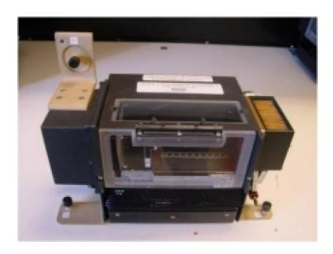
This is experiment hardware used by BASS. Samples are installed inside and a fan provides air to the flame. Credit: NASA
