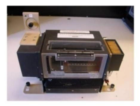
This is experiment hardware used by BASS. Samples are installed inside and a fan provides air to the flame. Credit: NASA
