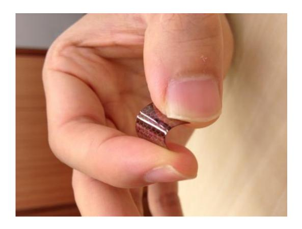
The flexible transparent electrode - "Flextrode."
