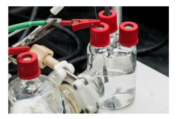
A UD engineering research team led by Feng Jiao has developed a highly selective catalyst capable of electrochemically converting carbon dioxide to carbon monoxide with 92 percent efficiency. Credit: Evan Krape
