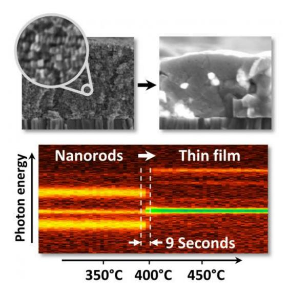
The transformation from a layer of closely packed nanorods (top left) to a polycrystalline semiconductor thin film (top right) can be observed in by in-situ X-ray diffraction in real time. The intensities of the diffraction signals are color coded in the image at the bottom. A detailed analysis of the signals reveals that
