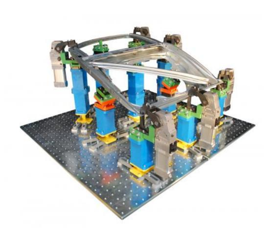
Clamping elements attach a metal part in car body assembly. A new device takes over the parameters set in the pilot production run, and makes the production process faster and more flexible. Credit: Fraunhofer IWU
