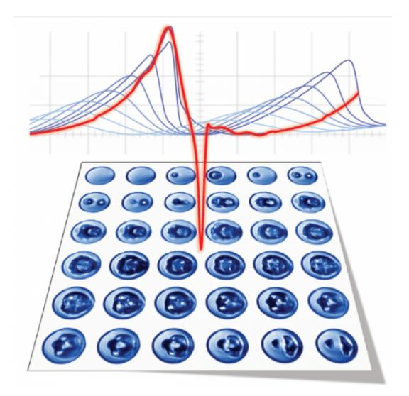
The ultrasound wave distorts to form a shock wave that is then focused within the drop. The highly focused ultrasound results in the vaporization of the drop, made visible here by Brandaris 128 high-speed imaging at a rate of 20 million frames per second (50 nanoseconds between each frame). Credit: PNAS
