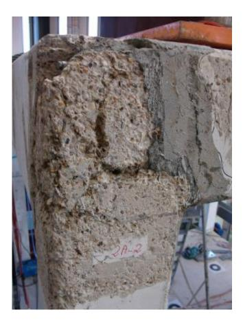
This is the same building joint, following application of post tensioned metal straps and tested on shaking table to equivalent of magnitude 7 earthquake. Credit: University of Sheffield
