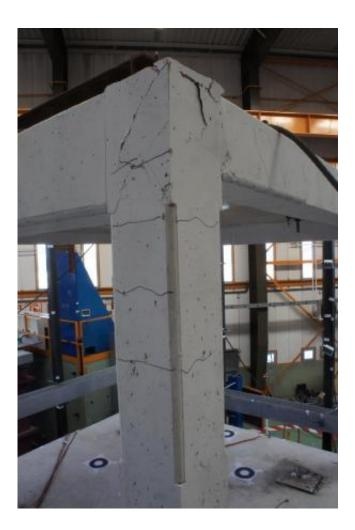
This is a damaged second floor building joint prior to testing with post tensioned metal straps. Credit: University of Sheffield
