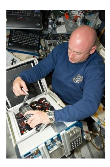
This is a view of STS-134 Commander Mark Kelly working with Group Activation Pack assemblies on the shuttle Flight Deck. Credit: NASA
