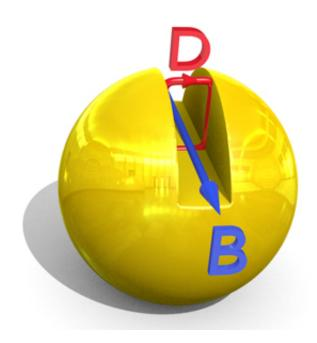
Meta-atoms comprising a metal nanosphere with a precisely etched trench have the electric (D) and magnetic (B) properties that allow them to interact with both components of visible light. Credit: A\*STAR Data Storage Institute
