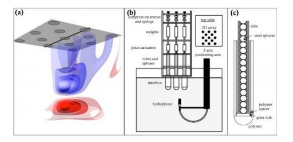
(a) Illustration of a sound bullet, where the surfaces are contours of constant pressure. The positive (red) and negative (blue) regions of the sound bullet are compact in 3D. (b) Experimental set-up of the acoustic lens, which is composed of 13 chains arranged in a square lattice. The hydrophone is used to measure sound under water. (c) Cross section of one of the chains and its casing. Credit: Donahue, et al. ©2014 AIP Publishing LLC
