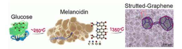
Scanning electron microscopy images for showing sugar blowing process: glucose were polymerized and blown by released ammonia into melanoidin bubbles in heating, which bubbles were finally converted into strutted graphene containing mono-/few-layered graphene membranes and graphitic struts.
