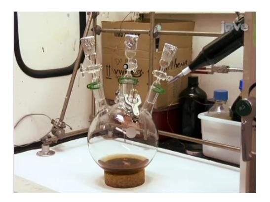
After a week of sparking in a Miller-Urey experiment, the contents within the reactant flask become visibly transformed. Miller-Urey's groundbreaking work is considered to be the first deliberate, efficient synthesis of biomolecules under simulated primitive Earth conditions. Credit: *The Journal of Visualized Experiments*
