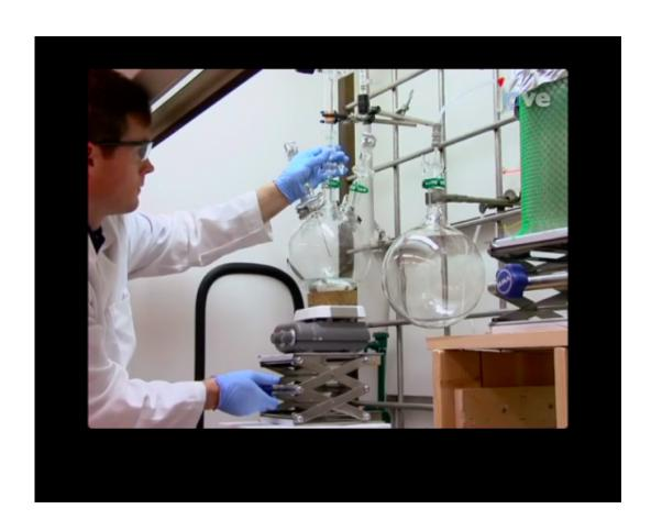
Miller-Urey experiments study the abiotic synthesis of organic compounds by creating an environment similar to that of the early earth. An electric discharge is applied to a mixture of gases representing the early earth's atmosphere and lightening. This is done in the presence of a liquid water reservoir, representing the early oceans, as well as with an apparatus simulating evaporation and precipitation. Credit: *The Journal of Visualized Experiments*
